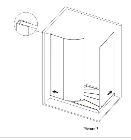
3. put the whole set of pull pole in the top of the glass in balance after assembling it , then put the pull pole connector to the wall and line the position in the wall. as picture 4
